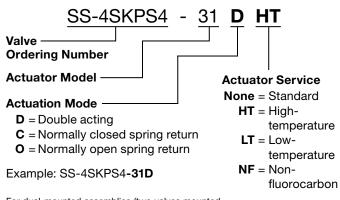
For dual-mounted assemblies (two valves mounted to one actuator), insert **DM** into the ordering number. Example: SS-4SKPS4-31D**DM**HT
