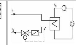
سمت بالا و قسمت خروجی نیز مقداری به Install a strainer at the input of the valve to prevent wastes and fillings of fluid inside it. While balancing برجهت جریان راداشته باشد ) تا از تجمع the steam line, pay attention that input side must be a little upper than output side to prevent accumulation of condense. While valve installation get assure that it must be horizontal and operating element must be installed vertical and downside.
