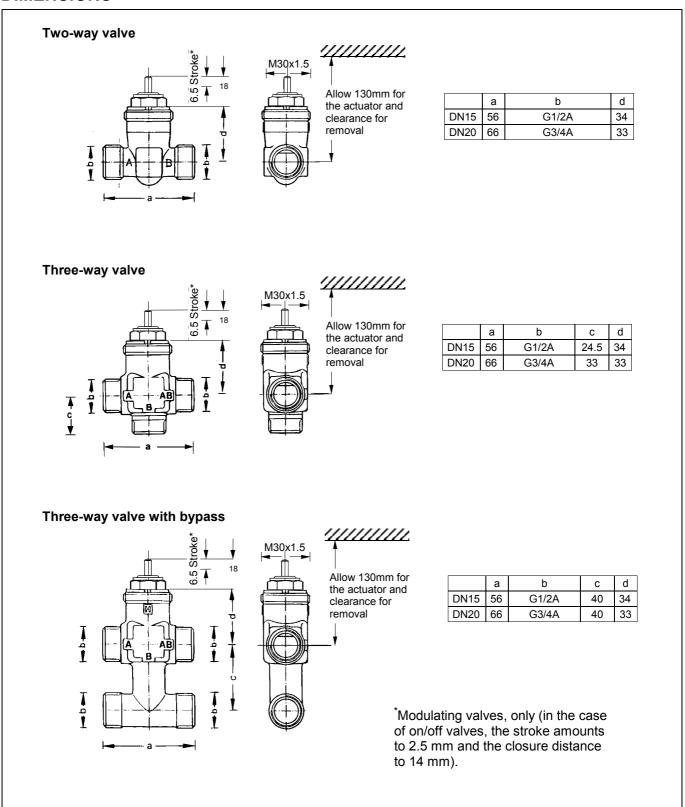
Fig. 4. Dimensions V5832A/V5833A,C in mm
