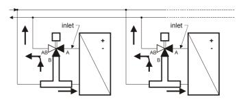
Fig. 3. Three-way valve with bypass
