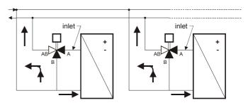
Fig. 2. Three-way valve operation
