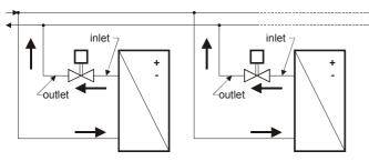
Fig. 1. Two-way valve operation
