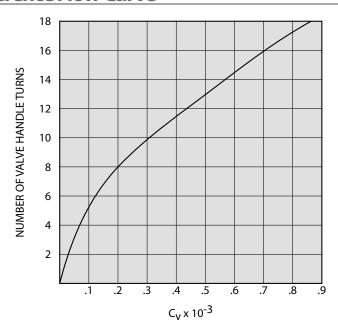
Metering range is approximately 18 handle turns. Opening the valve beyond the metering range will increase the flow to full Cv.
