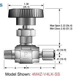
Panel Hole Diameter: 0.52 (13.2) Max Panel Thickness: 0.25 (6.4) Max Open 2.22 (56.4)
