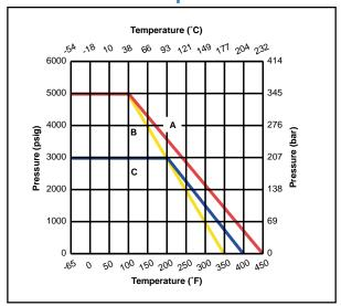
**Legend:** A - Stainless Steel with N or R stems; B - Stainless Steel with K stem; C - Brass, Steel, and Alloy 400 with N or R stems. Maximum temperature for Steel is 350 °F (177 °C)
